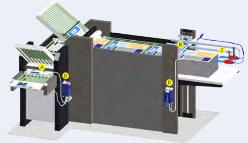
A Anti-static bars B Anti-static bar C Ionising nozzles D Power unit
