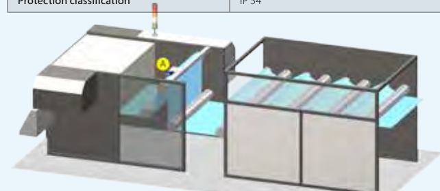
A Perfomaster; perforation detection and counting on a bagmaking machine
