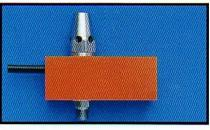
HS Nozzles are "shockless". The term shockless indicates that the ionizing point, located inside the nozzle tip, is capacitively coupled to the high voltage source, limiting the current at the point to a very low level. Under normal conditions, direct contact with the point will not
