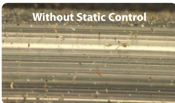
Catheter manufacturing after thirty (30) minutes of exposure.
